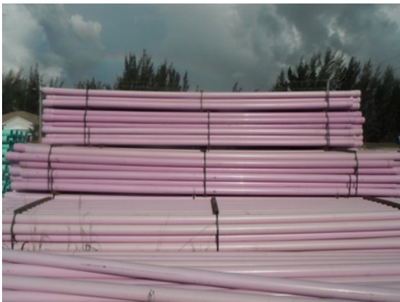
Irrigation Pipes (Purple Color Pipes)
